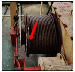
Figure 2 - Poorly- spooled Remote Control Wire.
