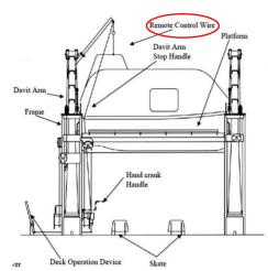
Figure 1 - Davit Launched Lifeboat Arrangement.
